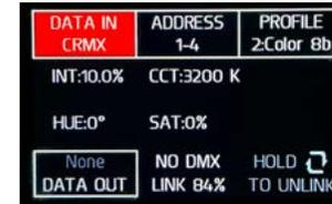
To unlink CRMX when in receiving mode, press the NAVIGATION button for 3 seconds (long press) while the data IN box is selected (when it is red).
