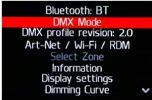
To use the MIX in ArtNet or DMX, go to SETTINGS \ DMX MODE. If you have plugged in a DMX cable, the light will go to DMX mode automatically.
