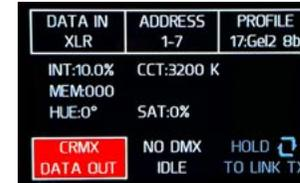
To link receivers when sending CRMX, press the NAVIGATION button for 3 seconds (long press) while the data OUT box is selected (when it is red).
