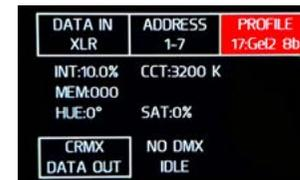
To unlink receivers when sending CRMX, press the NAVIGATION button for 3 seconds (long press) while neither the data IN nor OUT boxes are selected (in red).
